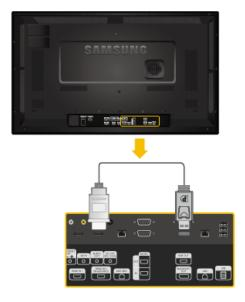
Connect the [MAGICINFO OUT] terminal and the [HDMI IN 2 (MAGICINFO)] terminal on the product using the DP to HDMI cable.
